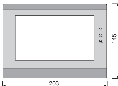
Centralized Control Panel Front Panel Physical Dimensions
